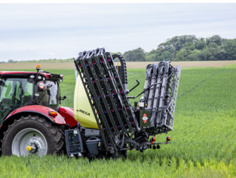
AutoFold for quick and secure boom folding.
