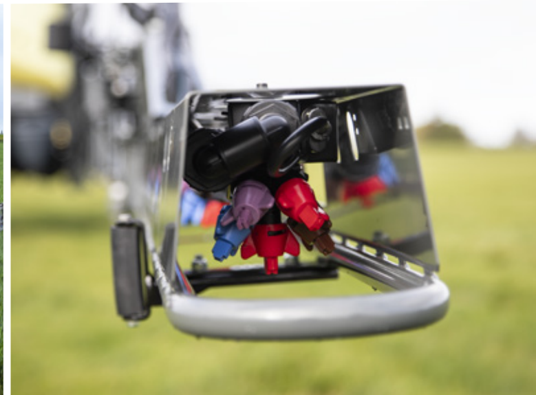
Nozzles protected for lower boom height and better drift control.
