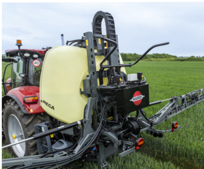
Long boom lift, for a large span of boom working heights from 50-210 cm.
